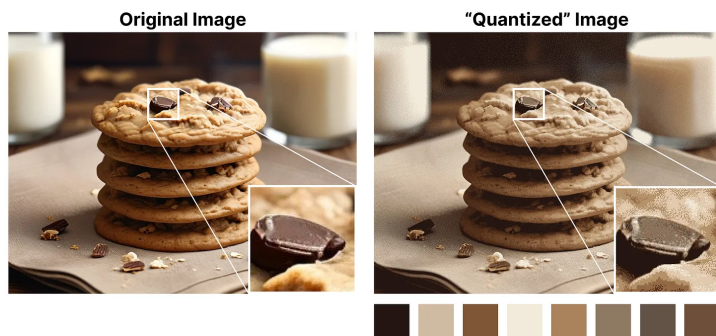
Figure 4: Quantization process illustration.
